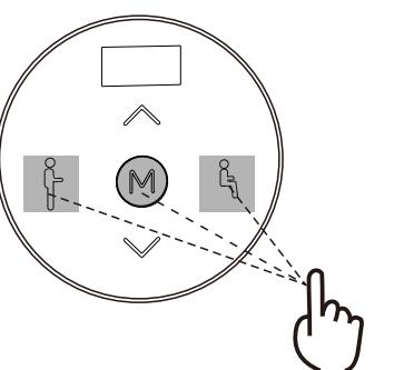
a. Press the up or down key to adjust the table to the required height, press M to save, and the display displays "S-"; Press "𠂇" or "𠂇" again to save the height to the corresponding position 1 or 2, and the corresponding display displays "S-1" or "S-2".
