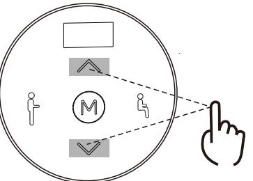
a. By pressing the "▼" or "▲" button, you can adjust the height of the lifting table up or down, and the current height will be displayed on the screen.
