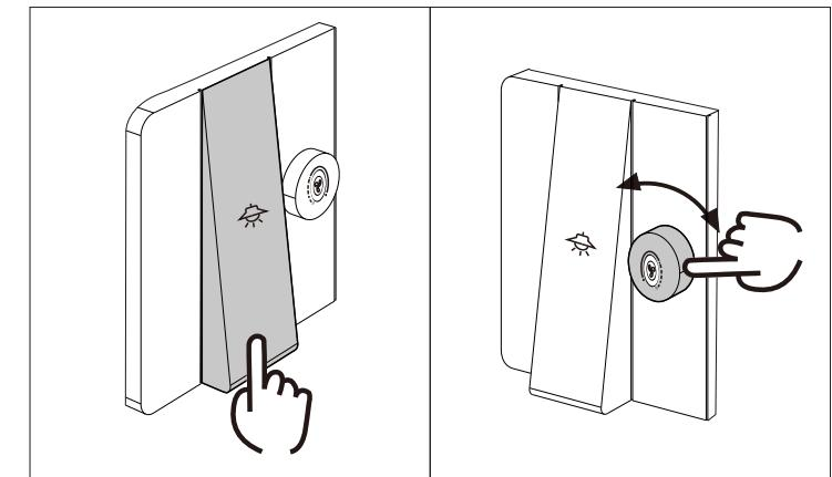
Click up and down to turn the light fixture on/off
