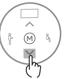
a. Reset function definition: The LED display shows "R51" or "R52". The user holds down the down arrow key until the desk lowers to the lowest position and then rebounds up to a stop. The display will show the lowest height. After releasing the "▼" down key, the reset is complete and the desk can be used normally again.
